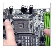
Visually inspect if the CPU is seated well into the socket. If not, take out the CPU with pure vertical motion and reinstall.
